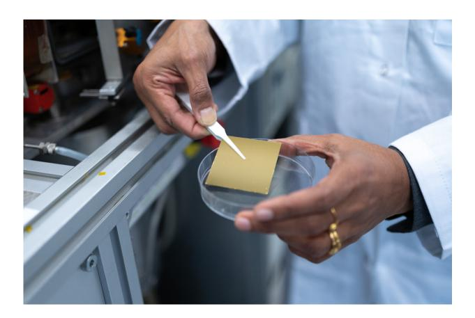
The two-dimensional silicon dioxide layer—not visible to the naked eye—is deposited on a gold surface. Credit: RUB, Kramer
