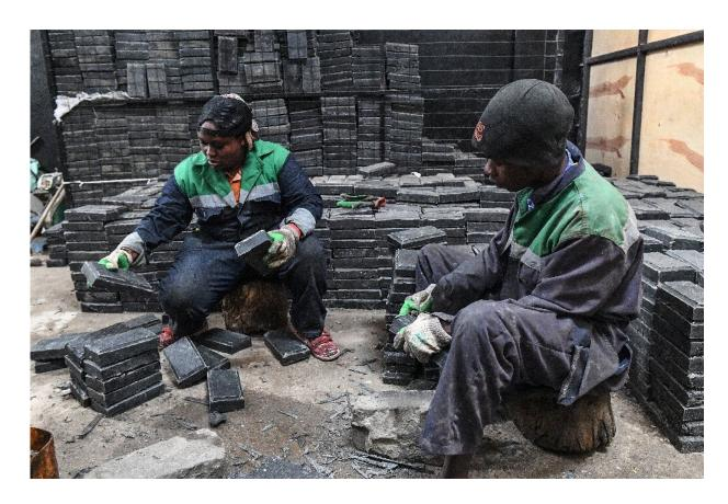
Every day, at their factory in Nairobi, Gjenge Makers churn out 1,500 bricks made from plastic trash that otherwise would be dumped in the city's overflowing garbage heaps.
