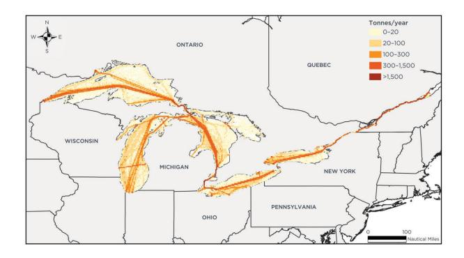
CO<sub>2</sub> emissions from ships in the GL-SLS in 2019. Created with AIS data from exactEarth, ship characteristics data from IHS Markit, and base maps from ArcGIS Online. Credit: ICCT
