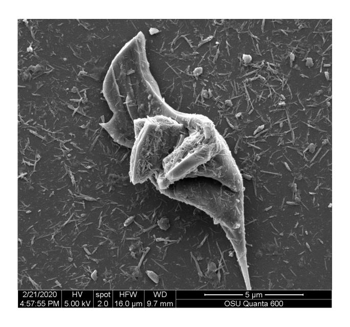
Scanning electron micrograph of tire particles after cryomilling tire tread. Larger particle is representative of micro-sized tire particles and smaller ones are nano-
