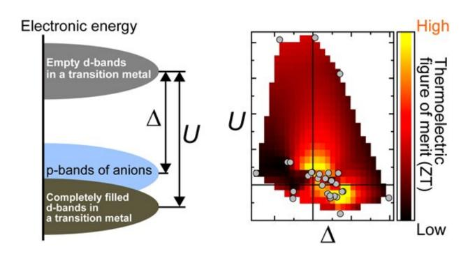
(Left) Schematic diagram explaining two electronic structure parameters: charge transfer energy ( $\Delta$ ) and onsite Coulomb repulsion energy (U). (Right) Plot of  $\Delta$  and U values indicating areas in which materials with desirable thermoelectric conversion properties can be found. Credit: Isao Ohkubo / National Institute for Materials Science
