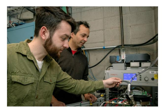
Will Larsen and Arun Persaud at the neutron test facility of the Fusion Science and Ion Beam Technology Program in the Accelerator Technology & Applied Physics Division, configuring the alpha particle detector. The alpha detector allows the measurement of the distribution of carbon atoms in soil. Credit: Berkeley Lab
