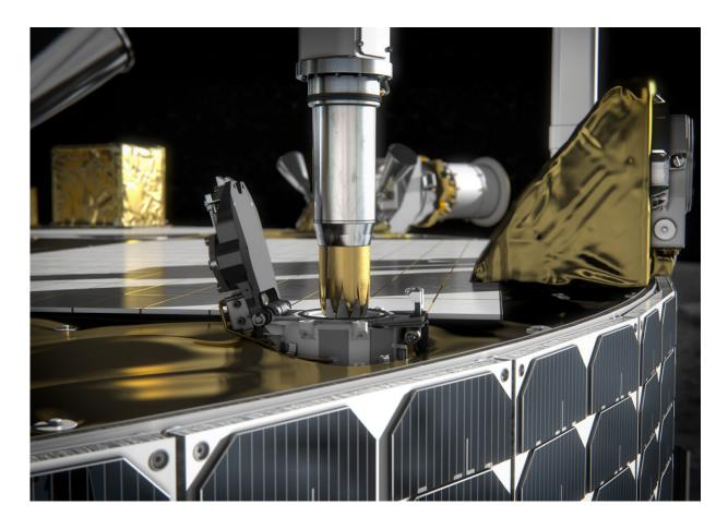
An artist impression of Lunar Lander collecting a sample on the moon. One task for Lunar Lander's scientific instruments will be to investigate Moon dust. A robotic arm will retrieve samples for closer inspection under an onboard microscope. Images and data will be sent back to Earth for further analysis. Credit: ESA
