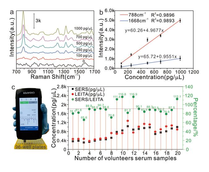
Figure 2. Detection of 5-fluorouracil in serum by hand-held Raman spectrometer. Credit: Zhou Guoliang
