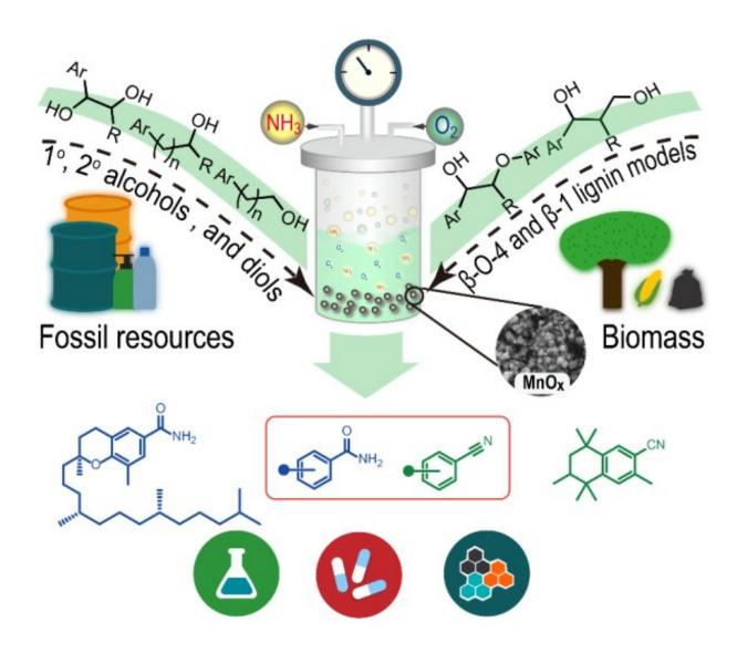
Schematic illustrations of the manganese oxide for catalytic cleavage and functionalization of alcohols reaction. Credit: He Peipei
