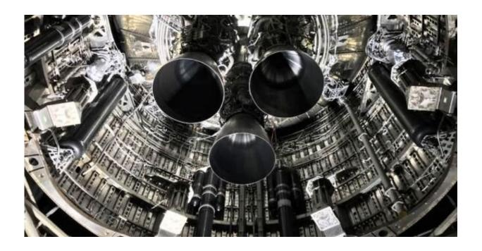
The engine compartment of the Starship, showing three Raptor engines. Credit: SpaceX
