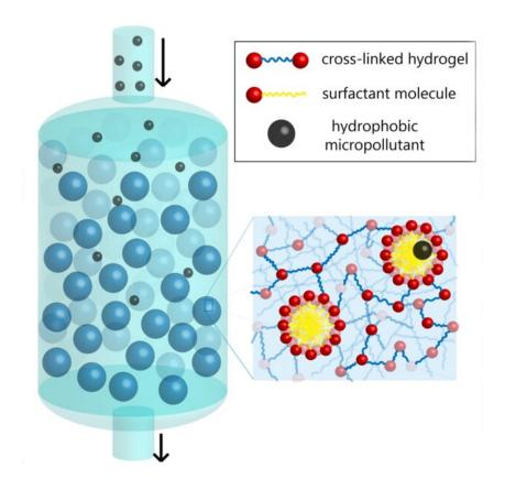
Caption:Schematic diagram of micelle-laden hydrogel particles in a packed bed for the removal of micropollutants. Credit: Doyle Lab
