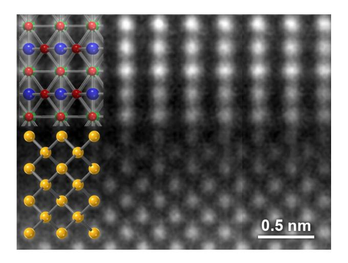
Scanning transmission electron micrograph of the interface between germanium (bottom) and LSZTO (top). The individual atoms are labeled gold: germanium, red: oxygen, green: strontium and lanthanum, blue: titanium and zirconium. Credit: Scott Chambers | Pacific Northwest National Laboratory
