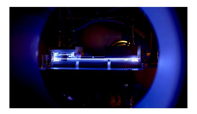
The two FLASHForward plasma cells observed through a vacuum window. The cells are filled with argon gas and then ionised with a high-voltage electrical discharge to form a plasma. As the plasma recombines it emits light in the blue wavelength range. Both plasma cells, of length 50 and 195 millimetres, can then be used for plasma acceleration of electron bunches in gigavolt-per-metre accelerating gradients. Credit: DESY, C.A. Lindstrøm
