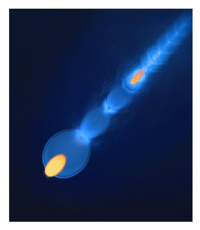
The novel diagnostic technique developed to enable this result relies on a pair of electron bunches (top right) interacting with the plasma perturbed by the leading bunch (bottom left). The recovery time of the plasma is defined as the separation between these two bunches at which the properties of the trailing electron-bunch
