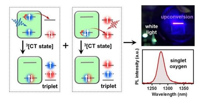
White-light-driven triplet-fusion photon upconversion and singlet oxygen generation by using nanocrystals to flip the spins to generate molecular triplets. Credit: *Chem* (2022). DOI: 10.1016/j.chempr.2022.03.003
