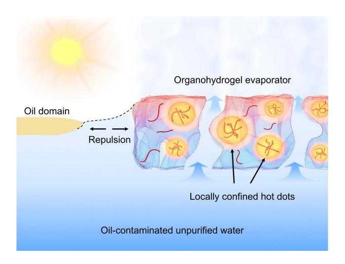
We propose an organogel-hydrogel compositing strategy for optimizing comprehensive performances of solar-driven evaporators in practical oil-polluted water purification. Ultra-stable floating ability, anti-oil-fouling property, accelerated vaporization process, long-term salt-resistance and scalability are integrated at one platform. Credit: *Nano Research* (2022). DOI: 10.1007/s12274-022-4118-8
