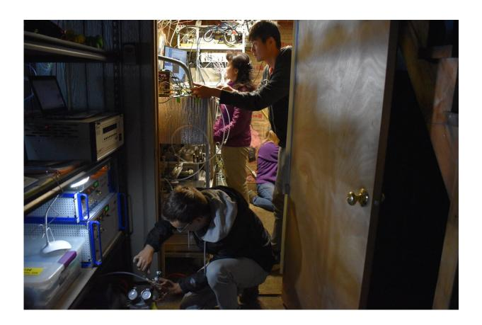
The UC Davis team sets up instruments for real-time ambient sampling at the Mount Bachelor Observatory in Oregon. Graduate student Christopher Niedek (front) sets up a particle generation system while Qi Zhang (middle) tunes a Soot Particle Aerosol Mass Spectrometer and graduate student Peng Sun works on the sampling line. Credit: Ryan Farley/UC Davis
