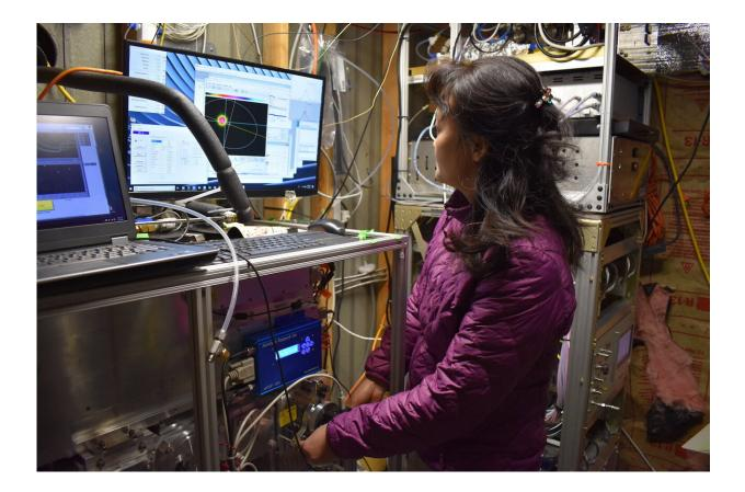
UC Davis Professor Qi Zhang tunes a laser vaporizer on the Soot Particle Aerosol Mass Spectrometer at Mount Bachelor Observatory to optimize detection for black carbon-containing particles. Credit: Christopher Niedek/UC Davis
