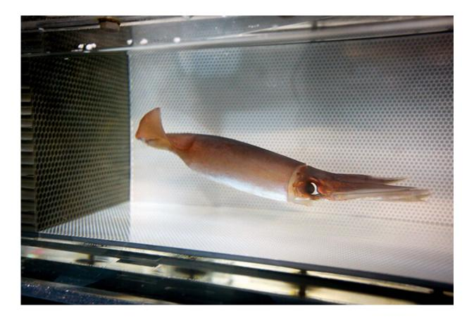
The jumbo squid, or Dosidicus gigas, inside a swim tunnel respirometer onboard a research ship. Seibel's team can control the water flow and have the squid swim against a current so they can measure their active metabolic rates. Credit: Stephani Gordon, Open Boat Films
