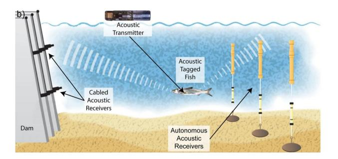
Schematic showing the key JSATS components of cabled acoustic receivers, autonomous acoustic receivers, and acoustic transmitters. Credit: Pacific Northwest National Laboratory
