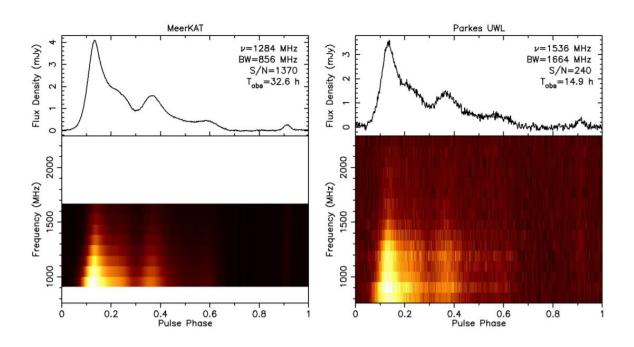
PSR J0955–6150: Flux calibrated total intensity profiles made from observations made with MeerKAT (left plot) and Parkes (right plot) radio telescopes. Credit: Serylak et al., 2022.
