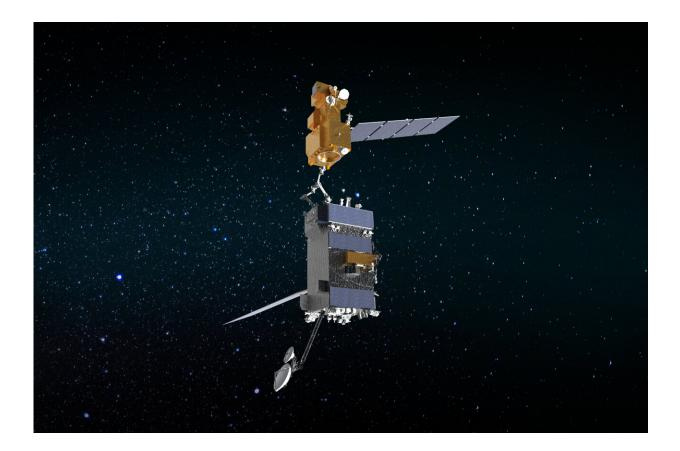
Illustration of OSAM-1 (bottom) grappling Landsat 7. Credit: NASA
