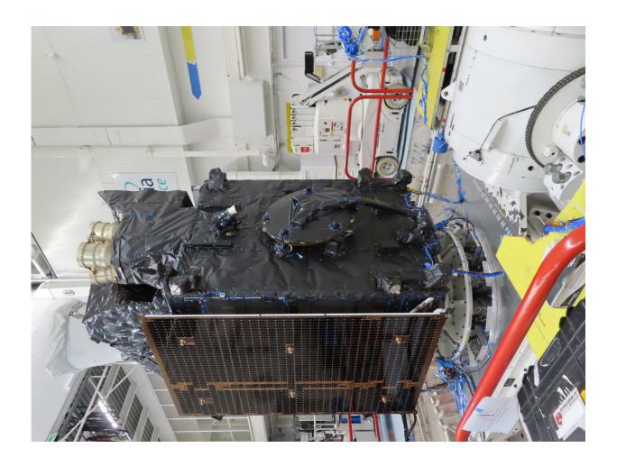
In preparation for liftoff, the first Meteosat Third Generation Imager satellite has been put through its paces at Thales Alenia Space's facilities in Cannes, France. With over 400 accelerometer lines installed and checked out, and around two tonnes of simulated propellant loaded, the satellite was mounted onto the shaker and was shaken to 'within an inch of its life', simulating the rigours of launch. Credit: Thales Alenia Space
