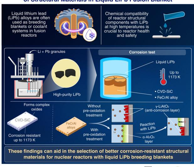
Corrosion-resistant materials for liquid LiPb fusion blanket in elevated temperature operation
