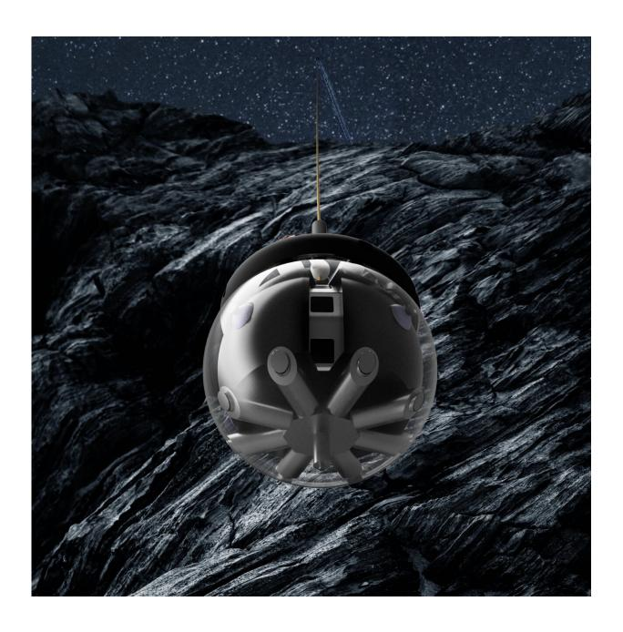
DAEDALUS would first be lowered into the cave mouth on a long tether, then disconnect to roll away autonomously under its own power. The hanging tether
