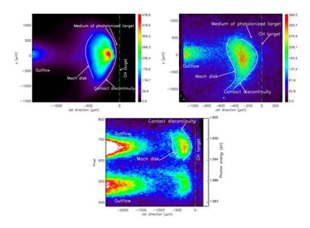
The X-ray morphology of the outflow and its interaction with a low-temperature medium from the photoionized CH target recorded using wide-field pinhole cameras with an energy band above 1 keV, and by an X-ray spectrometer with spatial resolution in the outflow direction. Left: due western (W) pinhole camera. Right: southeastern (SE) pinhole camera tilted to top. Bottom: due eastern (E)
