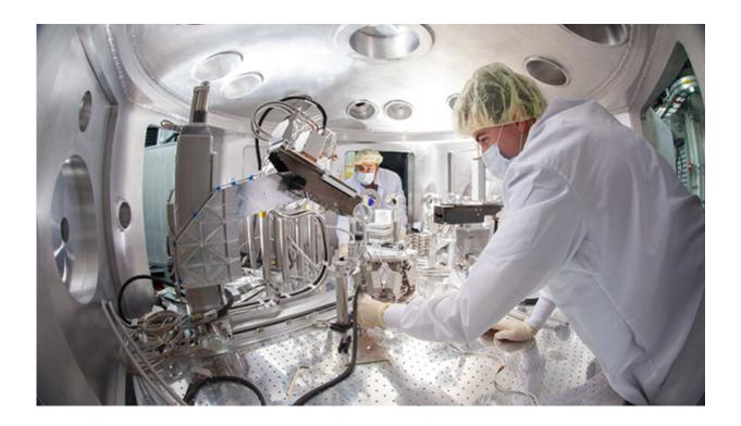
Researchers work in the "MEC hutch" of SLAC's LCLS Far Experiment Hall. The MEC optical laser system creates extreme temperatures and pressures in materials and the LCLS X-ray laser beam captures the material's response. Credit: Matt Beardsley/SLAC.
