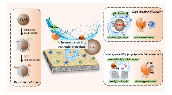
Preparation of reusable catalysts and schematics of the chemoenzymatic cascade reaction for cleaning polyamide NF membranes. Credit: ZHANG Jinxuan
