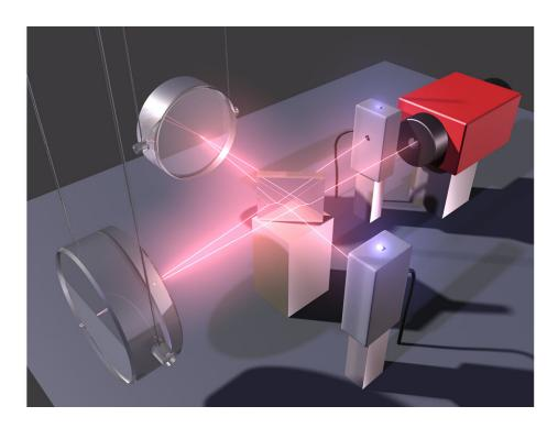
Schematic of a laser interferometer used to observe gravitational waves. If the quantum uncertainty of the radiation pressure of the light is the dominant dynamic force acting on the mirrors, a common quantum object arises from the mirror and the reflected light beam. In this case, the sensitivity of the interferometer is optimal when measuring changes in mirror positions due to gravitational waves. Credit: Alexander Franzen
