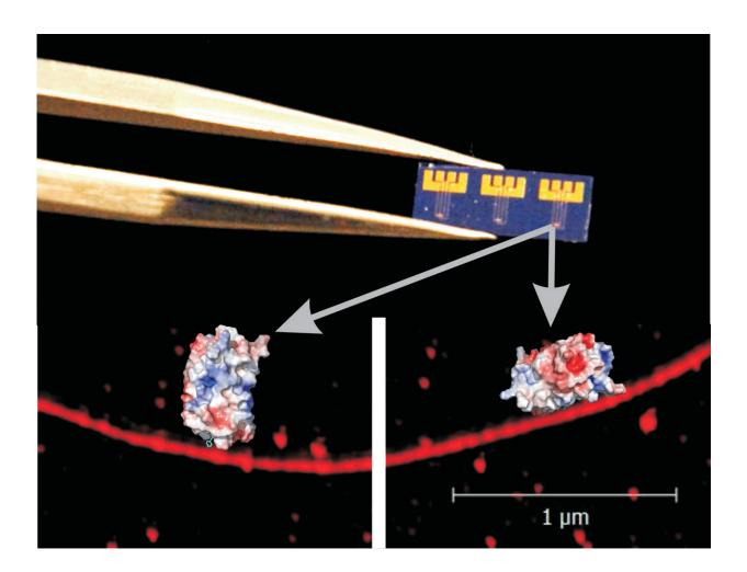
Chip with carbon nanotube transistor modified with green fluorescent protein with different attachment sites. Credit: MIET
