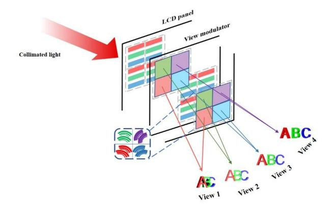
The researchers carefully designed diffractive flat lenses that were then intertwined to create a pixelated view modulator, the optical component that creates the various perspectives for a scene in a light field display. A 3D display that creates four views like the one pictured would incorporate four of these lenses, each of which converges the light into a unique view. Credit: Wen Qiao, Soochow University
