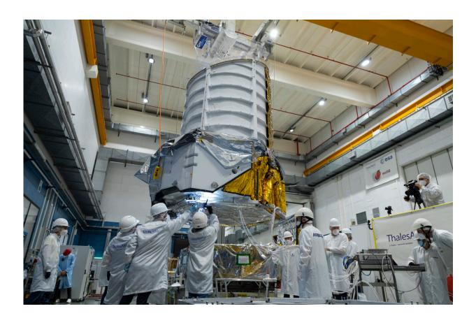
On 24 March 2022, ESA came one step closer to unveiling the mysteries of the dark Universe, following the coming together of two key parts of the Euclid spacecraft—the instrument-carrying payload module and the supporting service module. This image shows the 800-kilogram payload module being lifted by a crane, just before it was lowered onto the service module. Credit: ESA—S. Corvaja
