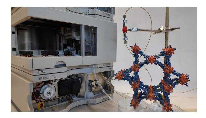
3D model of a MOF in front of the enzyme-MOF flow reactor at the laboratory of KIT's Institute of Functional Interfaces. Credit: Dr. Raphael Greifenstein, KIT
