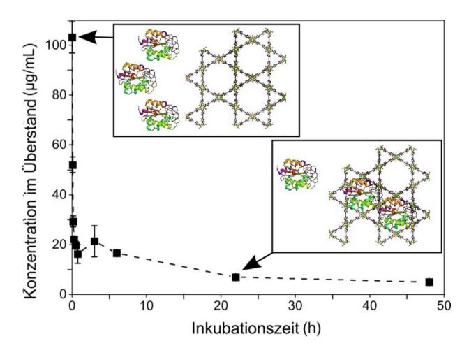
The huge biomolecules diffuse individually into the tightly fitting pores of a metal-organic framework. Credit: Dr. Raphael Greifenstein, KIT
