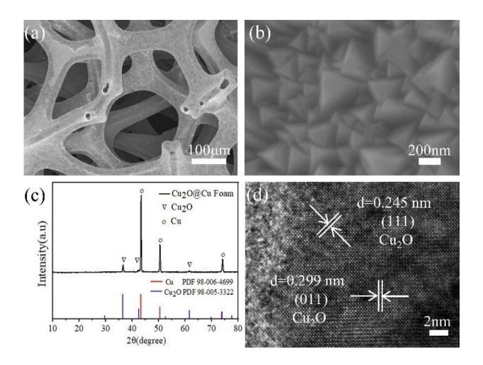
(a-b) SEM images and (c) XRD pattern of the electrodeposited  $Cu_2O$  thin films on frame of Cu foam; (d) HRTEM image of the as-prepared  $Cu_2O$  thin films. Credit: Tang Haibin
