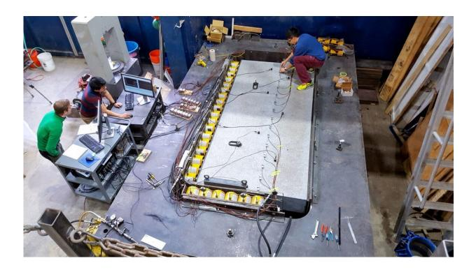
Stephan Schnabel, far left, a visitor from Sweden's Luleå University of Technology, Chun-Yu "Huey" Ke, Ph.D. '21, and Bill Wu, Ph.D. '21, prepare the Cornell 3m apparatus—that features a pair of two-ton slabs of granite—in the Bovay Lab for an earthquake experiment.
