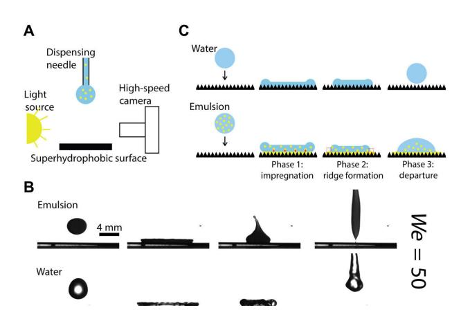
Impacts of water droplets and oil-in-water emulsion droplets on superhydrophobic surfaces. (A) Schematic of experimental setup. (B) Snapshots of high-speed videos of emulsion and water droplets impacting on a surface. The emulsion is a hexadecane-in-water emulsion at a concentration of 20%. At We = 50, both droplets bounce. At We = 87, water bounces while the emulsion sticks. At We = 95, both droplets splash and bounce. (C) Schematic of water and
