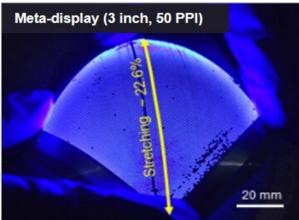
A 3-inch meta-display and a conventional stretchable display are attached to a hemispherical surface with a radius of 80 cm. The conventional stretchable display shows wrinkles and creases occur, but the meta-display is attached smoothly without any damage. Credit: The Korea Institute of Machinery and Materials (KIMM)
