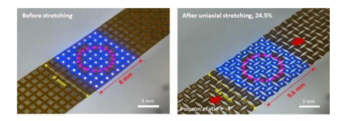
When the meta-display is stretched lengthwise, it is also stretched widthwise at the same ratio, so that the displayed image can be expanded without distortion. Credit: The Korea Institute of Machinery and Materials (KIMM)
