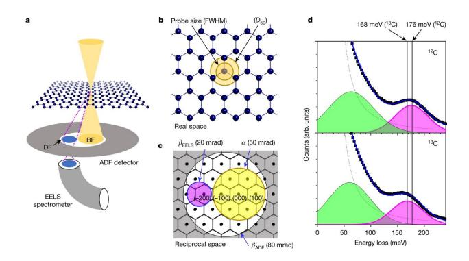
Fig. 1: Comparison of 12C and 13C graphene by dark-field EELS. Credit: *Nature* (2022). DOI: 10.1038/s41586-022-04405-w
