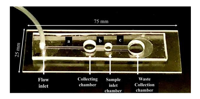
The microfluidic chip consists of four cylindrical chambers connected through microchannels: the fluid inlet chamber, collecting chamber, sample inlet chamber, and waste collection chamber. Credit: Florida Atlantic University
