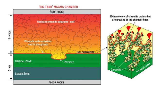
A 'big-tank' chamber of the Bushveld Complex (a) filled with a resident melt that crystallizes into the UG1 chromitite at the chamber floor as a 3D framework of touching chromite crystals (b). Credit: Wits University
