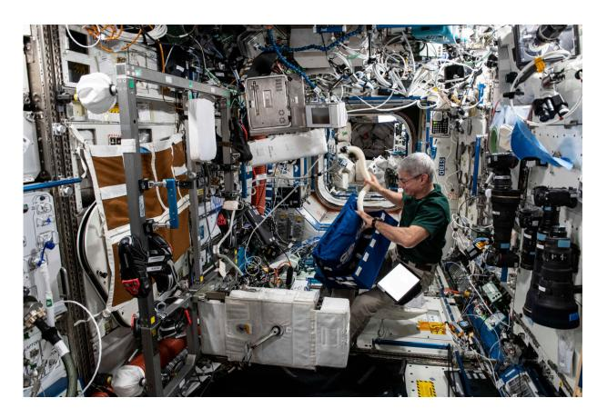
In this photo provided by NASA, astronaut and Expedition 65 Flight Engineer Mark Vande Hei sets up the International Space Station's exercise bicycle, also known as the Cycle Ergometer with Vibration Isolation and Stabilization (CEVIS), inside the U.S. Destiny laboratory module on June 22, 2021. Credit: NASA via AP
