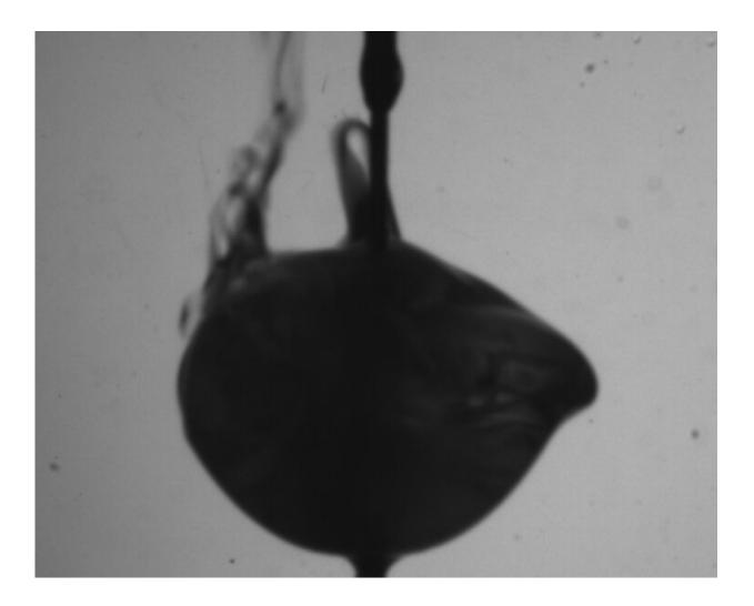
Water being released from a melting hailstone suspended in the air current of the wind tunnel. Credit: Alexander Theis
