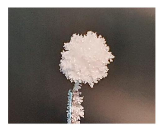
A rimed ice particle, in this case a graupel pellet, created for experimental use in the Mainz vertical wind tunnel. Credit: Alexander Theis
