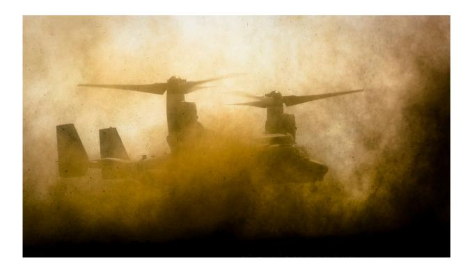
A U.S. Marine MV-22B Osprey lands at Babadag Training Area, Romania, in this 2015 photo illustration, kicking up clouds of potentially dangerous particulates in the process. Research at NPS employing the latest in Ultra High Temperature Ceramics has the potential to increase the resilience of turbine engines to particulate ingestion, critical for DOD aircraft operating in sandy and salty environments. Credit: U.S. Marine Corps photo illustration by Sgt. Paul Peterson
