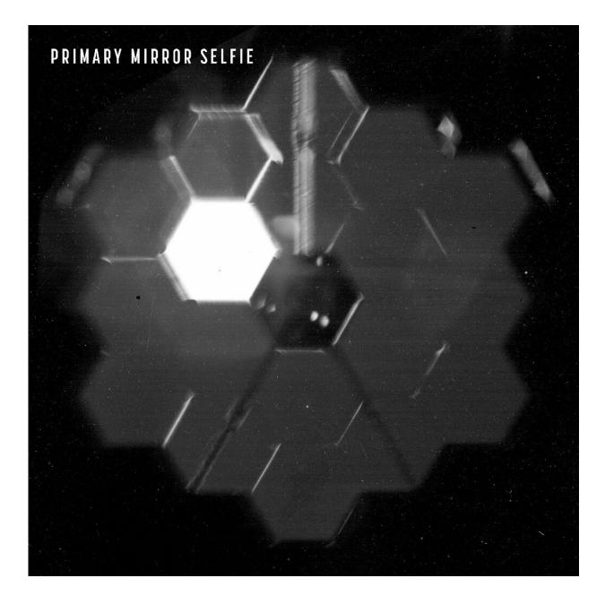
To aid the process, the team also captured a "selfie" taken not through an externally mounted camera but through a lens on board NIRCam.
