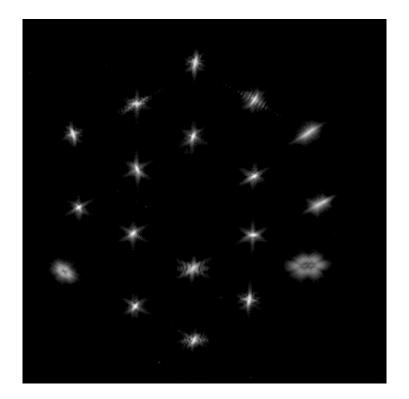
This gif shows the "before" and "after" images from segment alignment, when the team corrected large positioning errors of its primary mirror segments and updated the alignment of the secondary mirror. Credit: NASA/STScI
