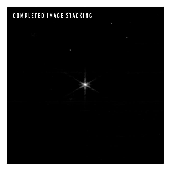
During this phase of alignment known as Image Stacking, individual segment images are moved so they fall precisely at the center of the field to produce one unified image instead of 18. In this image, all 18 segments are on top of each other. After future alignment steps, the image will be even sharper. Credit: NASA/STScI
