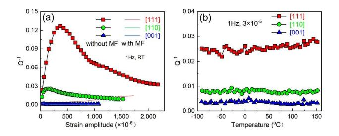
The variation of damping capacity with strain amplitude (a) and temperature (b) for [001]-, [110]-, and [111]-oriented single crystals at 1Hz. Credit: Sun Meng
