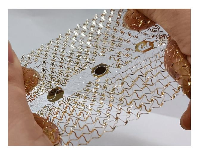
A stretchable "smart mesh" made from the two-mode cutting fabrication process. This device could be applied in skin-mounted sweat extraction and sensing. Credit: Peisheng He/UC Berkeley
