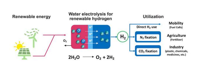
This schematic shows the concept for sustainable hydrogen production. Electricity from renewable sources (solar, wind) is used to split water into oxygen and hydrogen (electrolysis). The hydrogen can then be used for as fuel, to help make fertilizer from ammonia, and in other industries. Credit: RIKEN
