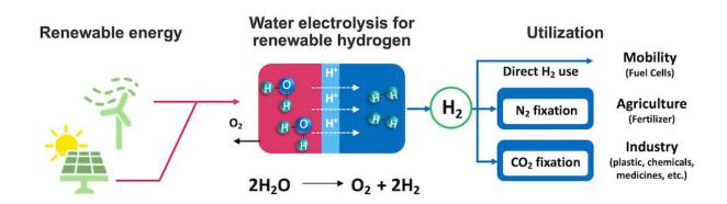
This schematic shows the concept for sustainable hydrogen production. Electricity from renewable sources (solar, wind) is used to split water into oxygen and hydrogen (electrolysis). The hydrogen can then be used for as fuel, to help make fertilizer from ammonia, and in other industries. Credit: RIKEN
