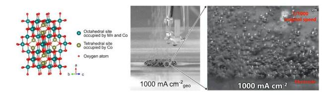
(Left) The mixed cobalt manganese oxide,  $Co_2MnO_4$ . (Right) a frame from a video showing hydrogen being produced through electrolysis at the current density of 1000 milliamperes per square centimeter. Credit: RIKEN
