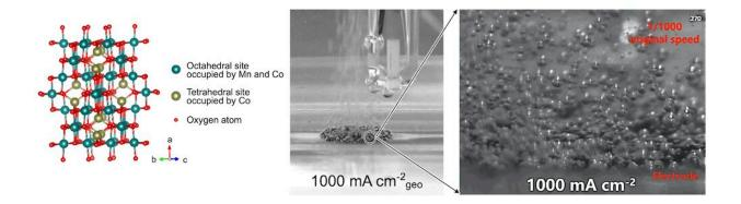
(Left) The mixed cobalt manganese oxide, Co<sub>2</sub>MnO<sub>4</sub>. (Right) a frame from a video showing hydrogen being produced through electrolysis at the current density of 1000 milliamperes per square centimeter. Credit: RIKEN
