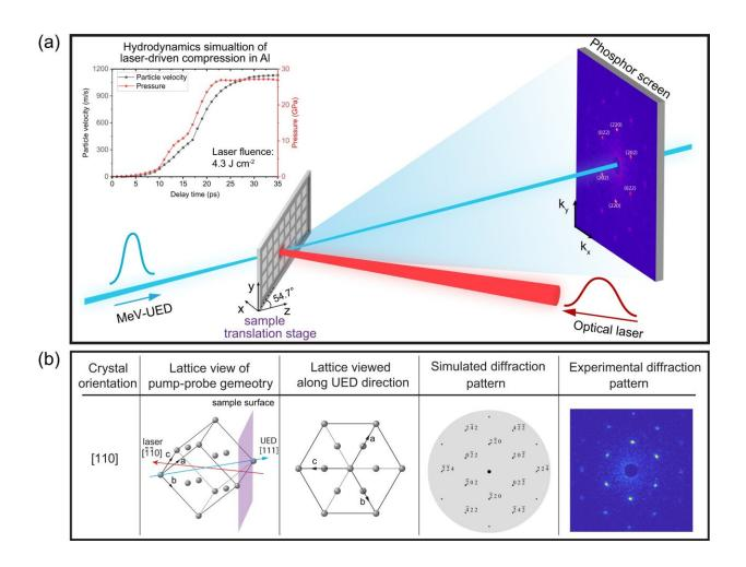
Fig. 1: Configuration for laser pump–electron probe experiments and diffraction patterns of Al single crystals at ambient (uncompressed) conditions. a Experimental setup for in situ UED under dynamic compression. The 3.7-MeV electrons generated by a radio-frequency (RF) gun are focused by two separate solenoids onto the sample; the electron beam spot size at the sample location is ~184  $\mu$ m × 250  $\mu$ m (x × y), the electron bunch charge is ~90 fC and the pulse
