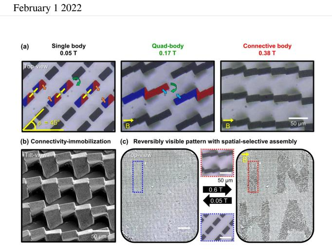
(a) Stepwise process of magnetic self-assembly at different magnetic flux densities (b) Polymeric binder allows shape-retention of long-range ordered connectivity after removal of magnetic field (c) Reversible appearance and disappearance of 'INHA' letters by spatial-selective assembly under an applied magnetic field. Credit: Inha University
