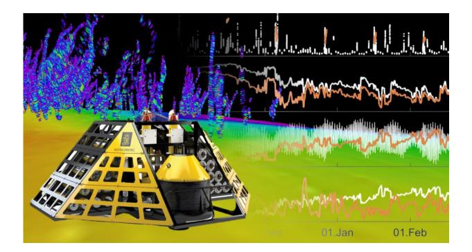
The K-lander observatory with a hydroacoustic collection of nearby bubble streams together with oceanic time-series data. Credit: Knut Ola Dølven and Manuel Moser (CAGE/UiT)
