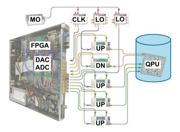
Diagram of QubiC prototype showing room-temperature electronics hardware. Credit: Gang Huang and Yilun/Berkeley Lab
