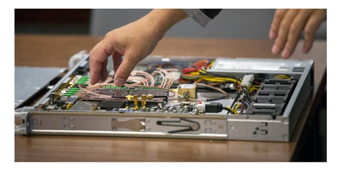
Researchers designed and open sourced a modular field-programmable gate array (FPGA)-based electronics control system called QubiC for superconducting quantum information processors. Credit: Berkeley Lab
